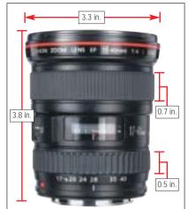
SPECIFICATIONS: 17–40mm (17.58–39.66mm tested), 14 (f/4.14–3.98 tested), 12 elements in 9 groups. Focusing turns 120 degrees counterclockwise. Zoom ring turns 60 degrees clockwise. Focal lengths marked at 17-, 20-, 24-, 28-, 35-, and 40mm. Diagonal View Angle: 104–57 degrees. Weight: 1 lb. Filter size: 77mm. Mount: Canon AF. Included: lenshood, soft case. List price: \$1,200. Street price: Approx. \$800.
